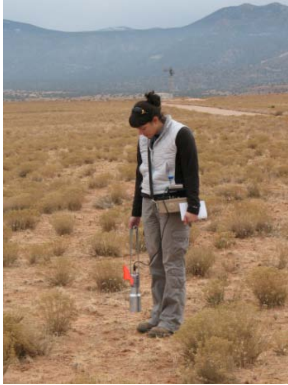
Photograph 5: Hand-Held 3-inch by 3-inch Sodium Iodide Detector
