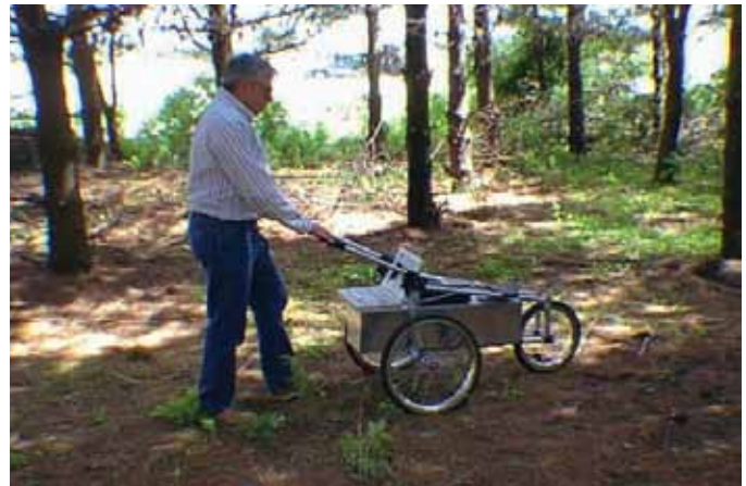
Cart with 4-inch by 4-inch by 16-inch Sodium Iodide Detector, one of several instruments USEPA will use to conduct the Gamma scan. It’s a small, maneuverable wheel-mounted transport system allowing access to some areas that will be cramped by rock outcrops or trees.
